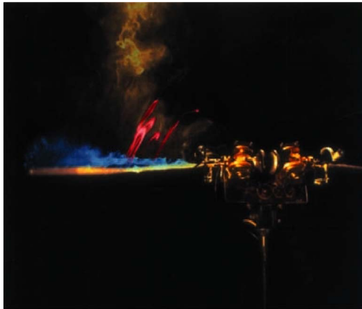
Fig. 10. Smoke visualization of the strong spanwise flow of the unsteady leading edge vortex (seen in blue). From Liu et al. [41].
