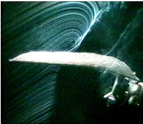
Fig. 12. The unsteady leading edge vortex as seen from behind and below a MAV wing. From Ho et al. [59].
