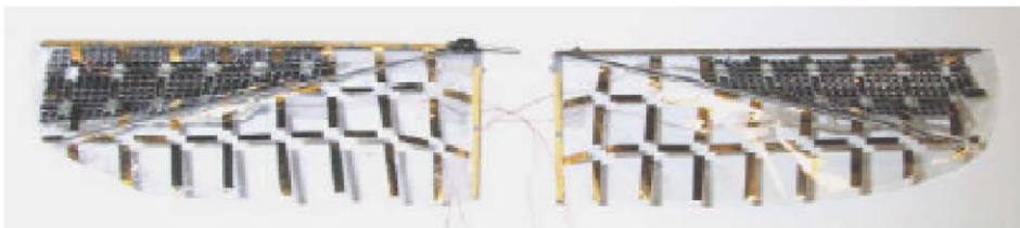
Fig. 25. Wing with integrated MEMS check-valve electrostatic actuators.
