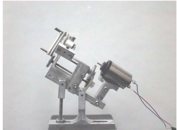
Fig. 32. DC motor and transmission system to flap wings.
