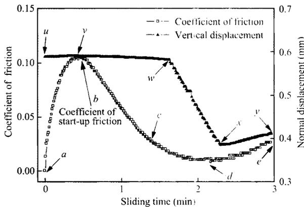
**Fig. 7** The coefficient of friction and normal displacement varying with sliding time, the sliding speed was  $4 \text{ mm}\cdot\text{s}^{-1}$  and loading time was 4 min.
