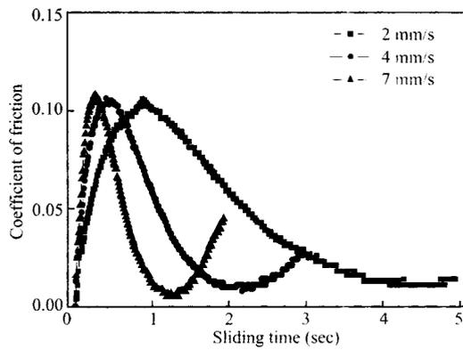
(b) The coefficient of friction as function of sliding time
