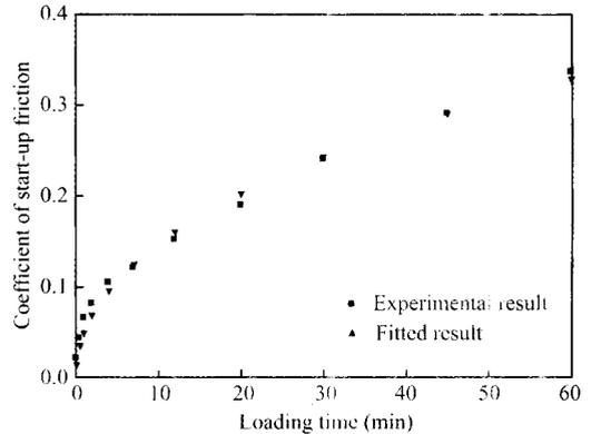
**Fig. 8** The coefficient of start-up friction and fitted results varying with loading time, sliding speed was  $4 \text{ mm}\cdot\text{s}^{-1}$ .
