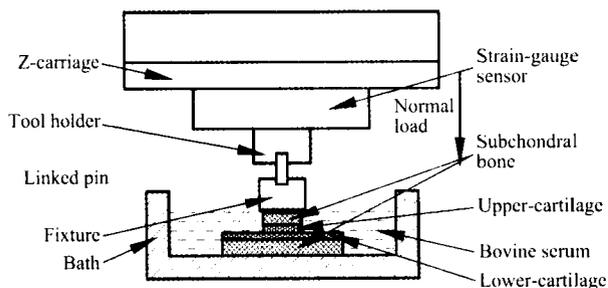
Fig. 1 Experimental methods of loading test of articular cartilage.
