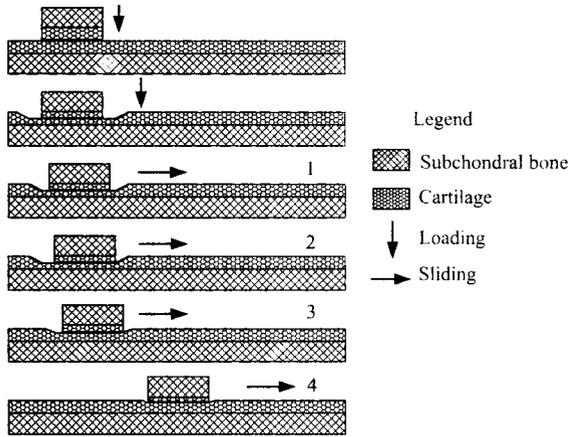
**Fig. 10 Normal displacements of upper cartilage and lower cartilage dynamically vary with sliding length.**
