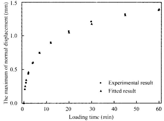
Fig. 5 Comparison of maximums of normal displacement and fitted results under different loading times.
