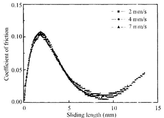
(a) The coefficient of friction as function of sliding length
