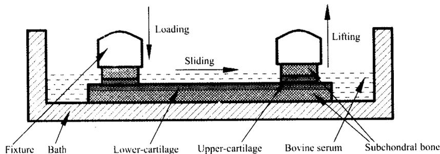
Fig. 2 Experimental methods of sliding test of articular cartilage.
