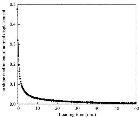
Fig. 4 The slope coefficient of normal displacement varied with loading time.
