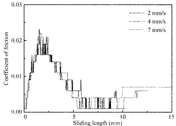
Fig. 6 The coefficient of friction as function of sliding length with different sliding speeds, loading time was 5 sec.
