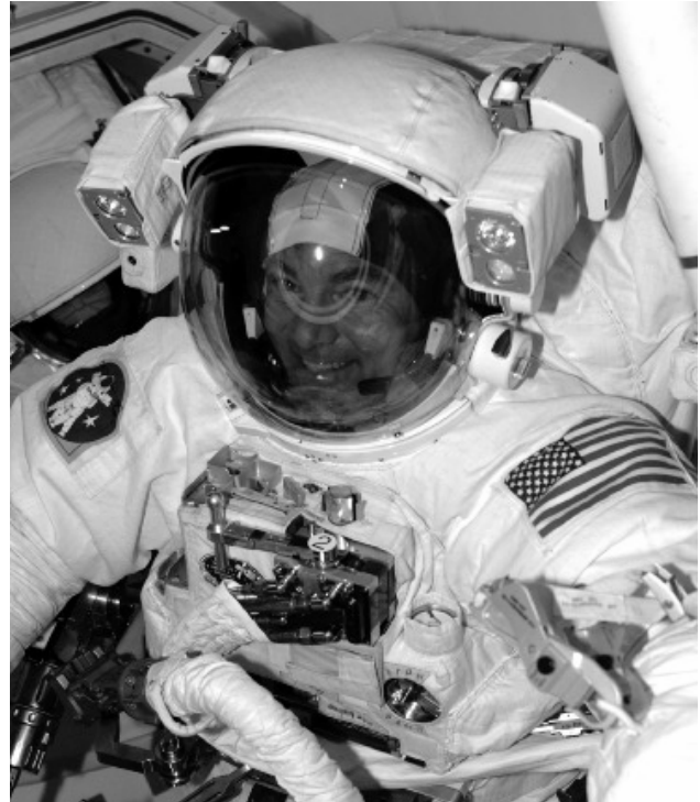
Figure 5. The chest mounted DCM provides accessible operator and vehicle interfaces.
