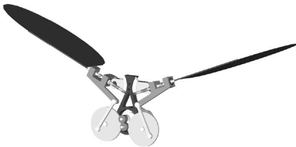
Fig. 2. AutoCAD illustration of the flapping wing micro air vehicle described in this paper, which is capable of achieving biaxial rotation of the wings using only a single electric motor.
