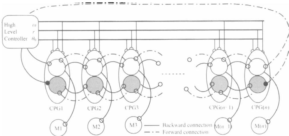
Fig. 5 Bionic neural network for fish-robot locomotion. The key parameters are controlled by the high level controller directly. The forward connections exist to transfer the propulsive wave from tail to head to make fish-robot swimming backward as soon as forward, just like what we observed in fish.
