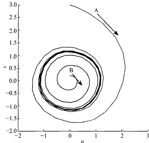
**Fig. 3** Limit cycles of Zhang oscillator in  $u-v$  phase plane, with  $k = 5$ ,  $r = 1$  and  $\omega = 2\pi$ .
