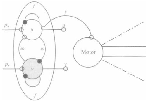
Fig. 4 Segmental CPG based on Zhang oscillator.
